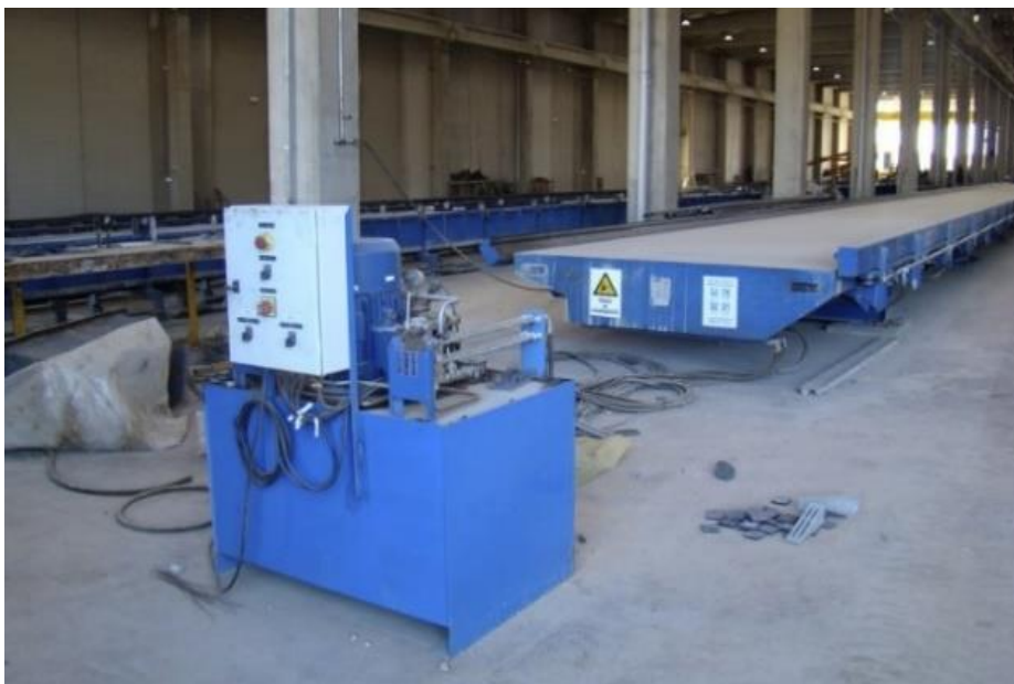
2-rasm. Panel ishlab chiqarish uchun zamonaviy universal rotor vibrostend.
